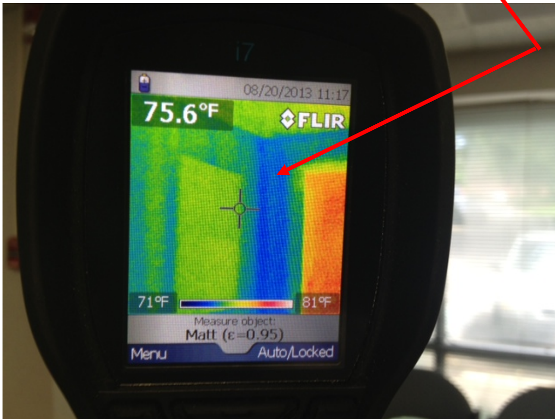
Thermal image of same area from previous photo. Heavy color contrast indicates there is no/poor insulation inside the wall cavity and no/poor protection from moisture pathways (i.e. vapor barrier).
